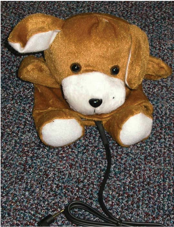
A Pal Pad inserted into a hand puppet becomes a soft, cuddly switch.
