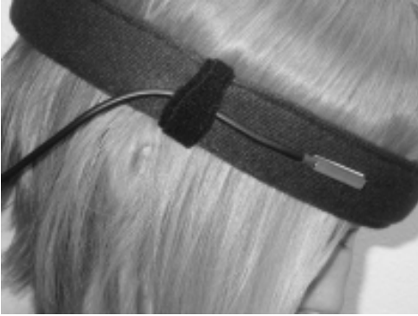
Tilting the head forward to a 30-degree angle will activate the Dipsy.
