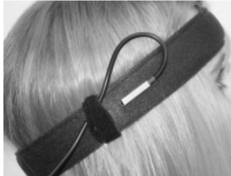
Tilting the head back to a 30-degree angle will activate the Dipsy.
